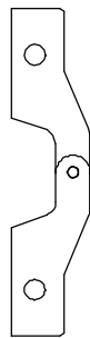
V-rig™ Flying Hinge for connection of cabinet front side, used both with V-rig™ LT and HD.
