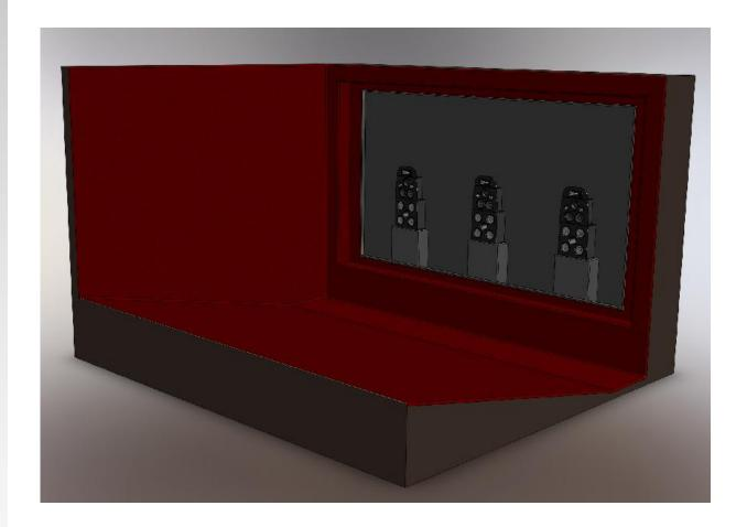
The Sound Projects X-perience is an ultra flat, flexible design cinema system consisting of three interchangeable modules: a subcabinet, a bas/mid cabinet of similar dimensions and a HF horn module. All parts can be interlocked for stability, allow flush mounting in a full baffle wall as well as precise vertical aiming to meet the most stringent criteria.
