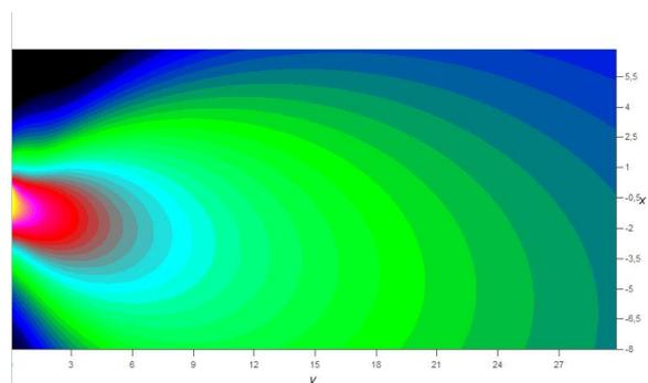
*Fig.1 Typical characteristic of a 2 meter array at 170 Hz.*
