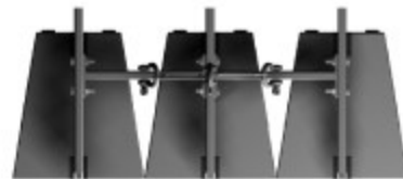
Top view of three arrays with 0-degree truss-to-truss connecting bars.
