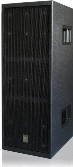
The sound reinforcement system shall hold two low-weight neodymium 15-inch drivers, powered by a 2500W class-D amplifier. The maximum peak output of the total system shall be 136dB at 1m. The system shall be switchable between full range or the 30-60Hz frequency range. The system coverage angle shall be omni-directional.
